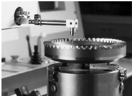
Computerized mapping of gear tooth profile
