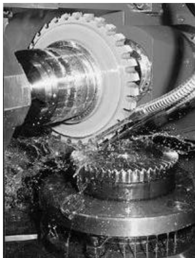
CNC machining of a PowerTRUE right-angle gear
